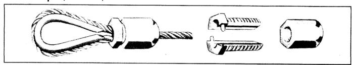
No more pressure! The Safe-Line Wire Rope Clamp is distributed by Esmet, Inc. These durable fittings are ideal for field installations that require quick, easily thimbled rope terminations, with the reliability that wire rope clips cannot provide. Designed only for 6 x 19 IWRC or 7 x 19 right regular-lay wire rope, the cadmium plated Safe-Line Clamp assembly includes a two-piece plug and cold-finish-bar steel socket.
